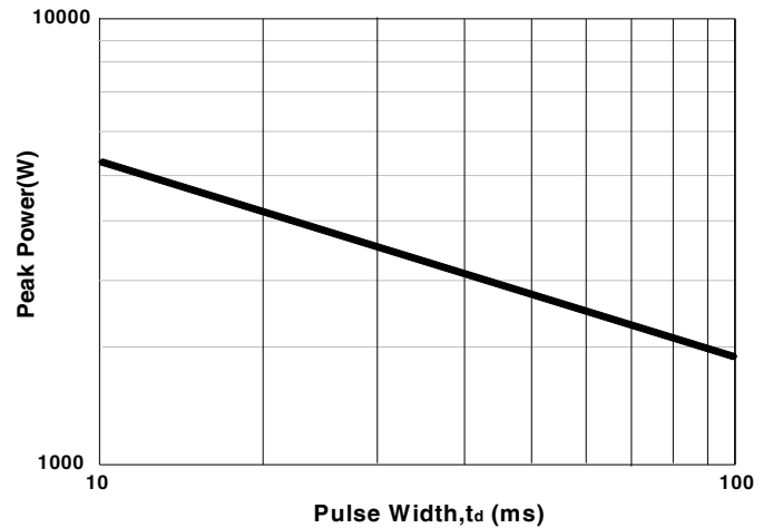
FIG.4 Peak Pulse Power Rating Curve
